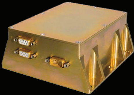
The JAVAD OEM GNSS board is embedded in the gle/RGU/G2T/HDA/MB1 for space missions. (Photo: GreenLake Engineering)
